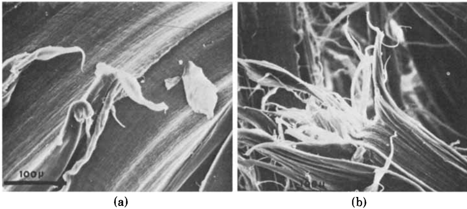
Fig. 13. Scanning electron micrographs of the failure surfaces of notched bars of Alathon 4275, deformed in (a) air and (b) isopropyl alcohol at a rate of 5.0 cm/min.
