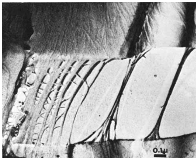
Fig. 21. Transmission electron micrograph of a thin film of melt-crystallized Alathon 4275 deposited on a carbon substrate on a Mylar strip. The Mylar was drawn 30%.
